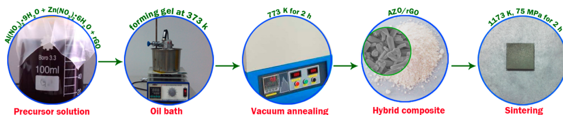
Figure 1. Schematic of the experimental procedure for preparing AZO/rGO hybrid materials.
